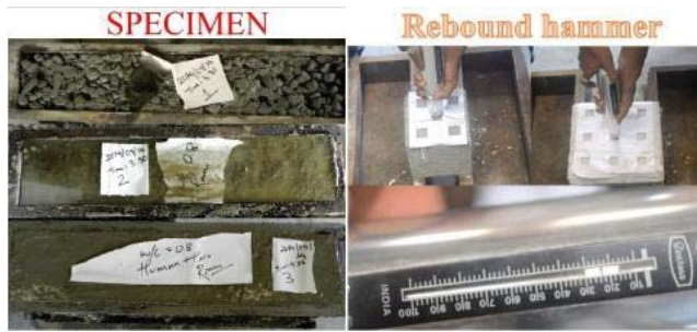
Fig 3 : Rebound hammer and Flexural test sample
